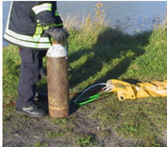
Filling the barrier from a compressed-air cylinder (300 bar).
