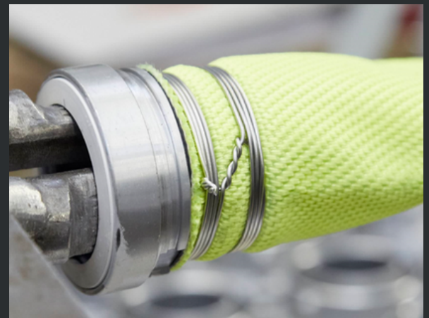
Wire binding of a Storz coupling
