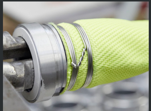
Wire binding of a Storz coupling
